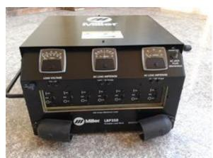
SANA had been considered one of the most famous companies in using a calibrated welding machines and what made it special in this field was clarified below: Calibrations performed by most other companies utilize a hand held clamp-on amp meter and standard volt meter and the readings are taken while the operator is welding at one output setting. We utilize a resistance load bank specifically designed to test and calibrate the output from welding machines.
